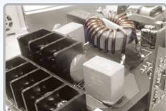
Built-in EMC Filter (C2 class)
