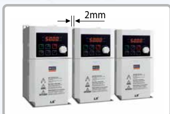
Side-by-side Installation (2mm between drives)
